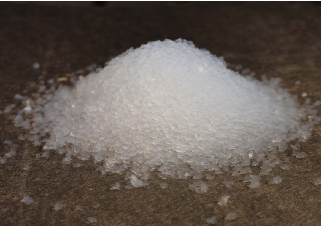
Basismaterial: 85% nanoporöses Aerogel
